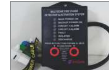
Driver operated manual control switch will function independently of vehicle power
