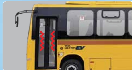
Pneumatic Door with Sensitivity for Passenger Safety#
